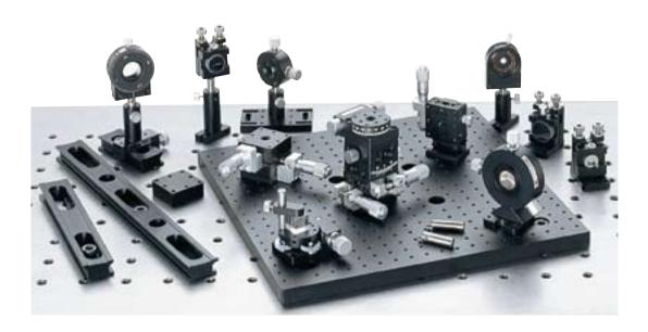
This system facilitates close stacking of components and the building of small scale optical systems assemblies. Holders are offered for 10mm and 15mm optics since these sizes lend themselves most effectively to diode and fiber systems. A system of mounts and rails permits the movement of components relative to each other.
