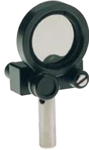
A mini-filter holder is offered here. It consists of a double clamp mounted on a rod. Filters may be mounted on either side of the rod simply by releasing the spring loaded clamp against the filter. This method is quite secure for filters which rarely need any critical positioning.
