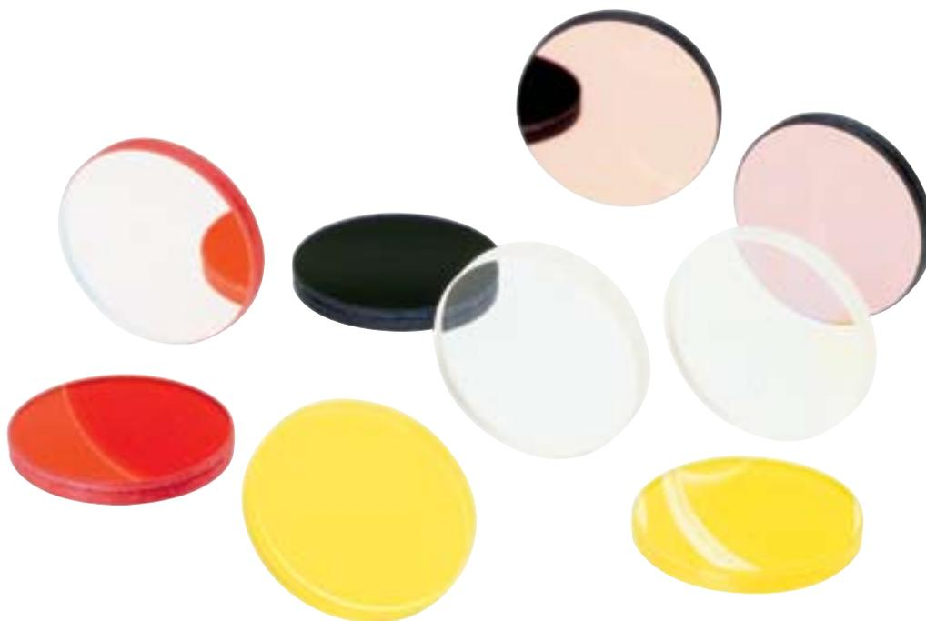
Edge filters may be tilt tuned just as narrowband filters. The specified center wavelength will shift 50nm towards the blue for increasing angles of incidence. All of these edge filters may be tuned from their center wavelength to the next lower wavelength range.
