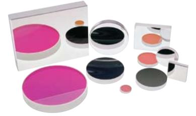
Mirrors are a critical and commonly used component in many optical systems. They are used to fold, bend and focus optical beams. They often allow a more compact and manageable system design. Optical quality mirrors are coated on their front surface with a metallic or dielectric coating to reflect the light. Three characteristics are important when choosing an optical mirror: surface figure, surface quality and the coating specification.
